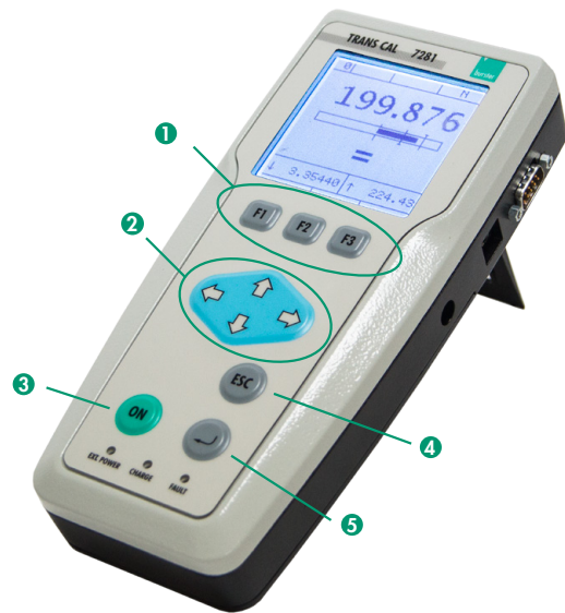
Diagram 3: Controls of TRANS CAL model 7281
