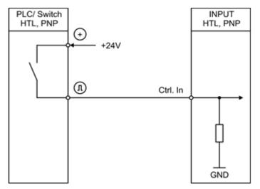
Open control inputs are "low active". The inputs could be used for control purposes. They could be used for different functions regarding the parameterization.
