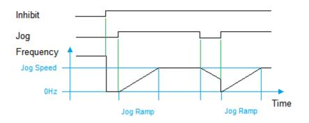
Process Jog: New setting of Jog before 0Hz are reached (Special Mode not equal to zero)
