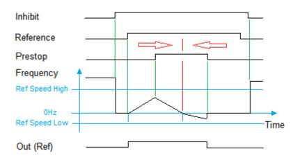
If the limit switch already appears during the ascending ramp, the frequency is then ramped down at the current position. If the limit switch already appears during the reverse ramp, the ramp is stopped at the current position.
