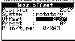
The offset is subtracted from the physical position. This makes it possible for you to shift the zero point.
