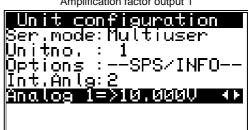
With keys and by you can set the amplification and the offset through repeated ajustments with the keys and measuring the analog output voltage. From analog output 1 to analog output 2 and to switch between offset and amplification factor, press keys , or CR. When all 4 adjustments are made, the input is ended with the CR key and the menu is left.
