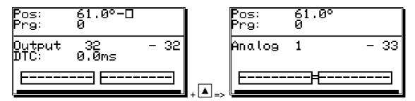
The output numbers of the analog cam outputs are always added to the numbers of "normal" outputs and this number can be selected directly from the programming menu. If you have configured e.g. 32 cam outputs, the number of the first analog cam starts at the output 33. The output number of the analog cam changes automatically when you change the number of "normal" outputs (see chapter "7.4.6.2. Setting the outputs" on page 62).
