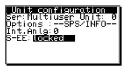
Therefore select **S-EE** in menu **"unit configuration"** and change it by pressing to **"locked"**. If the EEProm is locked, **all** data will only be written to RAM and will be deleted if the voltage is switched off.
