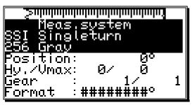
The display gives the resolution of the measuring system in steps per rotation. Generally the CamCon works with a rotation angle coder that has a resolution of 360 steps per rotation. In this case a change in the input value is superfluous. Otherwise the CamCon can be adjusted to the measuring system with the separate with the land keys. You can choose between the following predefined resolutions, that are all in accordance with
