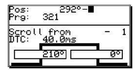
The upper part shows the current actual position, the switched state of the selected output and the chosen program. The lower part displays an output with programmed cams and their activation and their deactivation points. If no input is made within two minutes the CamCon automatically returns to the main menu for reasons of safety.
