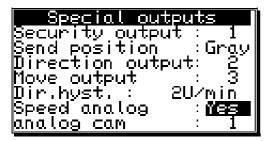
CamCon emitts a voltage (proportional to the speed) on the first analog output (pin 2 at CamCon DC50), 0 to -10V with a negative rotation direction and 0 to +10V with a positive rotation direction, if the menu point "Speed Analog" is set to "yes".
