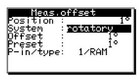
Here you can indicate, using the and keys, wether your controlling system is a rotatory (e.g. an eccentric press) or a linear (e.g. a knee lever press) moved system.
