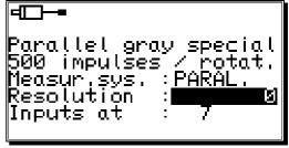
In our example the position of the LSB would be at input 7. With a resolution of 500 impulses 9 bits of resolution are needed. The CamCon automatically determines the position of the remaining inputs once it knows the position of the LSB; they are determined in increasing order. In our example inputs 7 to 16 would be allocated with the bits of the rotation encoder.
