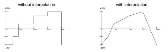
Through interpolation of the definition points, CamCon can adjust the values and present a curve, corresponding to the above right drawing.
