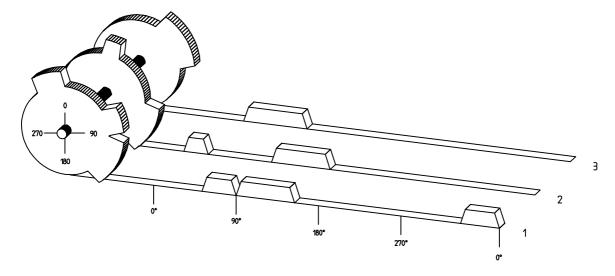
Diagram: Principles of a Cam Switch Unit
