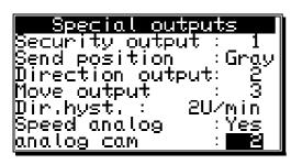
With a CamCon cam controller you have the possibillity to make an output of free programmable analog values (cams) dependent on the position. You enter the number of analog outputs in the menu point "Analog cams", that you want to program via the CamCon. In most cases, this will also be the number of your analog hardware outputs.
