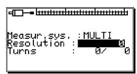
**Example 1:** You have a rotation plate with an electronic gear rate of 3 to 1, i.e. the encoder rotates 3 times for every rotation of the plate. These three rotations correspond with 360 impulses (360 degrees). You need to make the following inputs:
