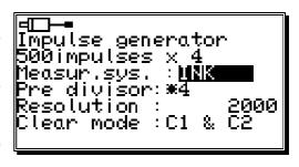
Here the prescaler is set to "\*4". This means that a measuring system with a resolution of 500 impulses supplies the device with 2000 impulses.
