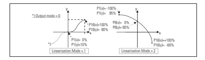
You can visualize your curve on the PC screen or by means of an external oscilloscope. For this, select TOOLS, then TEST and there "Analogue Voltage Function". The unit will now simulate a repeating counting cycle over the full range and generate the analog signal accordingly. When you use the Scope function of the operator software, you must set the serial code ":1" to record the analog output.
