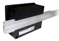
ELGO-Guide rails up to 2 m are already equipped with the necessary absolute encoded magnetic tape. The magnetic tape will be delivered separately if more than one guide rail is needed (measuring lengths longer than 2 m). Thanks to the absolute measuring method, no further referencing is necessary after setting the zero point once.
